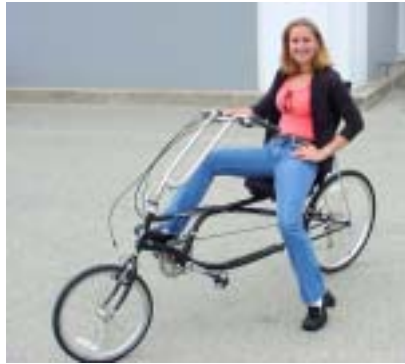
Figure 17: A USA long-wheelbase recumbent bicycle (from www.easyracers.com )
